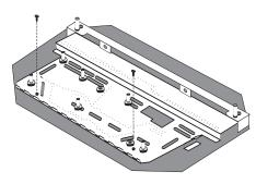
**10)** Remove all 18 screws holding the burner tray assembly in place.
